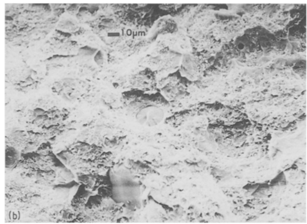
Figure 12 Fracture surface of a Zimmer LVC specimen shown in two magnifications. Note the density and the morphology of the secondary fractures in this material.
