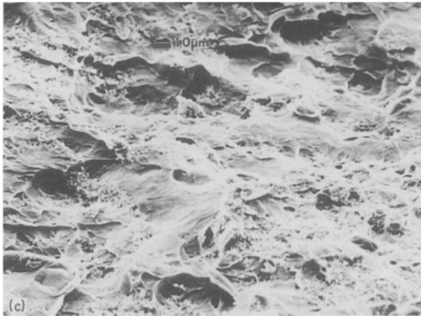
Figure 8 Medium magnification SEM fractographs of Zimmer LVC (a) UHM, (b) CHM and (c) CFG specimens. Note that at this magnification the three fracture surfaces are indistinguishable.
