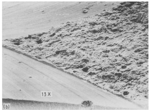
Figure 6 Low magnification SEM fractographs of Zimmer LVC (a) UHM, (b) CHM, and (c) CFG specimens. Note that the fracture surface of the UHM specimen is much less planar than the other two.
